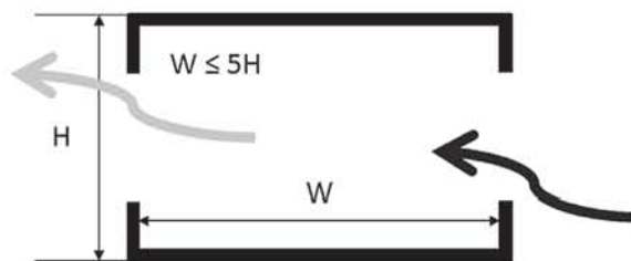
Figure 5.2 Schematic showing the principle of crossflow ventilation
